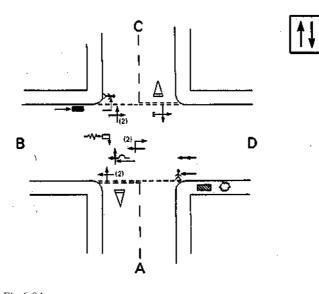
Fig 6.04 Typical collision diagram (ref 5)
