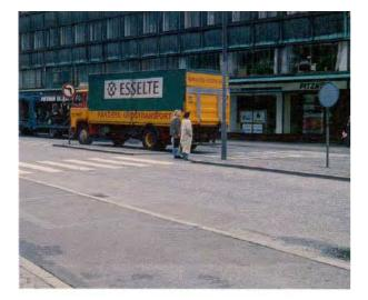
Fig 6.61 Zebra crossing in Denmark where central refuge provides a safe wafting area for pedestrians (TRL)
