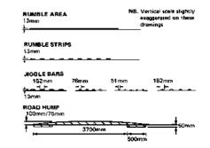
**Fig 6.44** Dimensioned sketches of speed reducing devices (ref 1 and 4)
