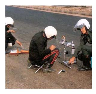
Fig 5.15 Police in Egypt using TRL portable device to measure skid resistance (TRL)
