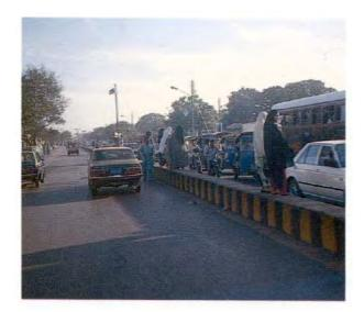
Fig 4.43 Narrow median barrier in Pakistan, separates traffic but creates dangers for pedestrians due to inadequate width (Ross Silcock Partnership)
