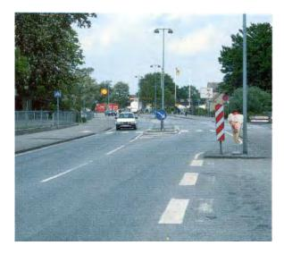
Fig 6.43 Lane narrowing and chicane used as a traffic calming (ie. speed reducing) device in Denmark (TRL)
