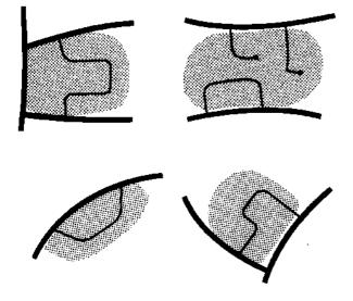
Fig 3.30 Examples of good layouts where through traffic is unlikely to use access roads (ref 10)
