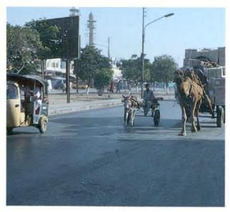
Fig 4.65 Slow-moving vehicles on a dual carriageway in Pakistan cause delays and potential conflicts with faster traffic (TRL)
