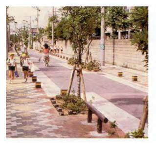
Fig 3.37 A Yuzuriha Street in Japan where pedestrians are given priority and speed reducing devices are used (City of Osaka)
