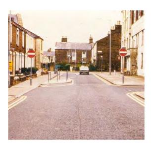
Fig 6.47 Half closure at intersection, UK (TRL)
