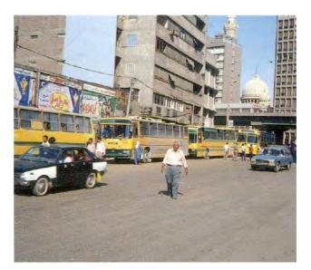
Fig 5.28 Absence of road markings on wide roadway in Egypt causes confusion and increases accident potential (Ross Silcock Partnership)
