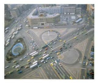
Fig 4.90 Painted road markings create effective channelisation on a large urban intersection in Korea
