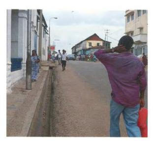
Fig 4.54 Inadequate footway width and street furniture obstructions force pedestrians to walk in road, Ghana (TRL)
