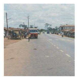
Fig 4.52 Ample space provided off-road for bus to pickup/drop passengers in Ghana. Note shaded bus shelter (TRL)
