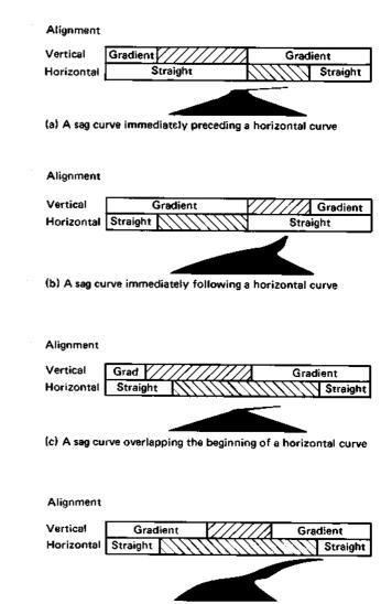
(d) A sag curve occurring within a horizontal curve
