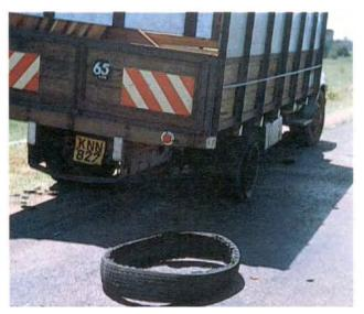
Fig 5.43 Dangerous tyre conditions on a goods vehicle in Kenya (Rendel Palmer & Tritton)
