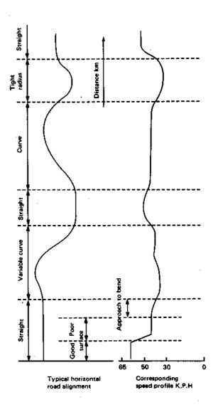
Fig 4.02 Schematic relationship between speed and horizontal curvature
