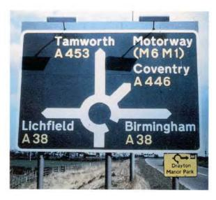
Fig 4.87 Map type direction sign also provides information about the type of intersection ahead in the UK (Ross Silcock Partnership)
