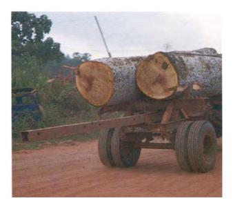
Fig 5.31 Dangerous vehicle in Ghana. Unmarked protruding metal bar is a danger to following traffic (TRL)
