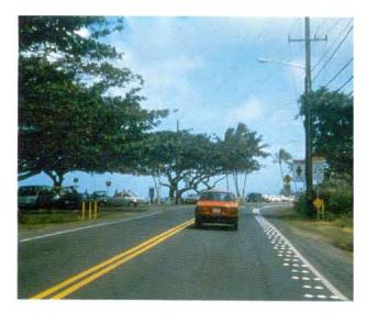
Fig 6.32 Double centre line to designate no overtaking and conspicuous edge marking to defuse tight curve. USA (Ministry of Construction, Korea)
