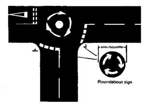
Fig 6.16 Poor roundabout layout: no deflection on entry thus traffic can pass through without slowing down (ref 3)
