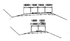
Cross-sections, particularly on roads in built-up areas, are often not uniform. Local developments may encroach onto the carriageway because of a lack of effective planning control. In rural conditions cross-sections may be reduced at drainage structures.
