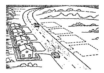
Fig 5.21 Individual houses have their own access onto a main road. New houses planned opposite will lead to further accident risk (ref 7)
