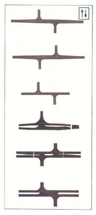
Fig 4.72 Typical Layouts of priority intersections showing UK practice and road markings (ref 3)
