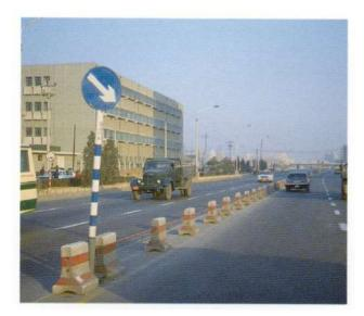
Fig 4.45 Movable concrete block and steel rail barrier in Chula, separates traffic and provides ease of relocation when required (Ross Silcock Partnership)
