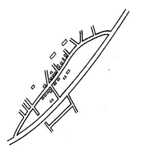
Fig 3.14 A bypass removes through traffic from the village in Fig 3.12. Note limited access points onto new road (Ross Silcock Partnership).
