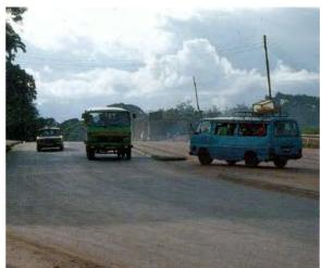
Fig 6.48 Illegal U-turns just over the brow of a hill have caused accident problems at this site in Ghana (TRL)
