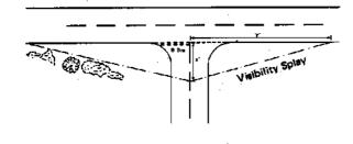
**Fig 4.82** Visibility splay on straight sections UK practice (ref 1)
