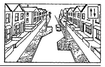
Fig 6.54 Chicanes with local road narrowing offer a means of reducing speeds and improving conditions for pedestians (UK Department of Transport)
