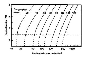
Fig 4.11 Superelevation design curves (ref 4)
